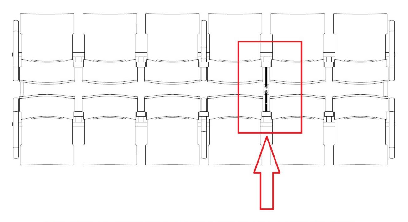
EXIT POINT OF CABLE (COVERED WITH 16MM PVC PROTECTIVE SLEEVE) FROM THE BOTTOM OF MAIN BEAM CAN BE PLACED IN ANY POSITION ON THE BEAM.
